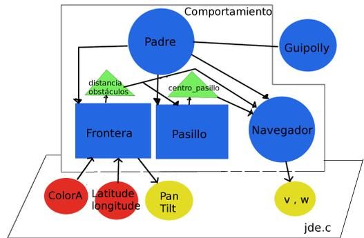
Figure 1: Schema design for the navigation behavior based on visual memory
