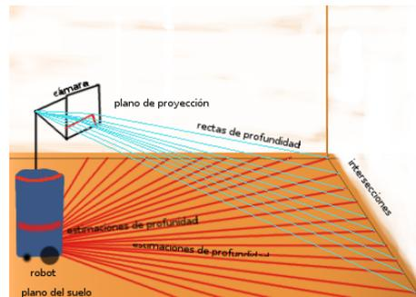
Figure 2: Depth from a monocular image
